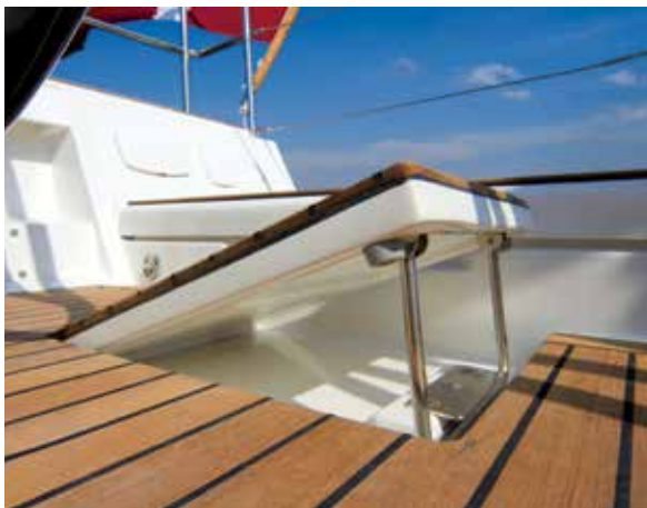
Top: Adjustable folding foot chocks
