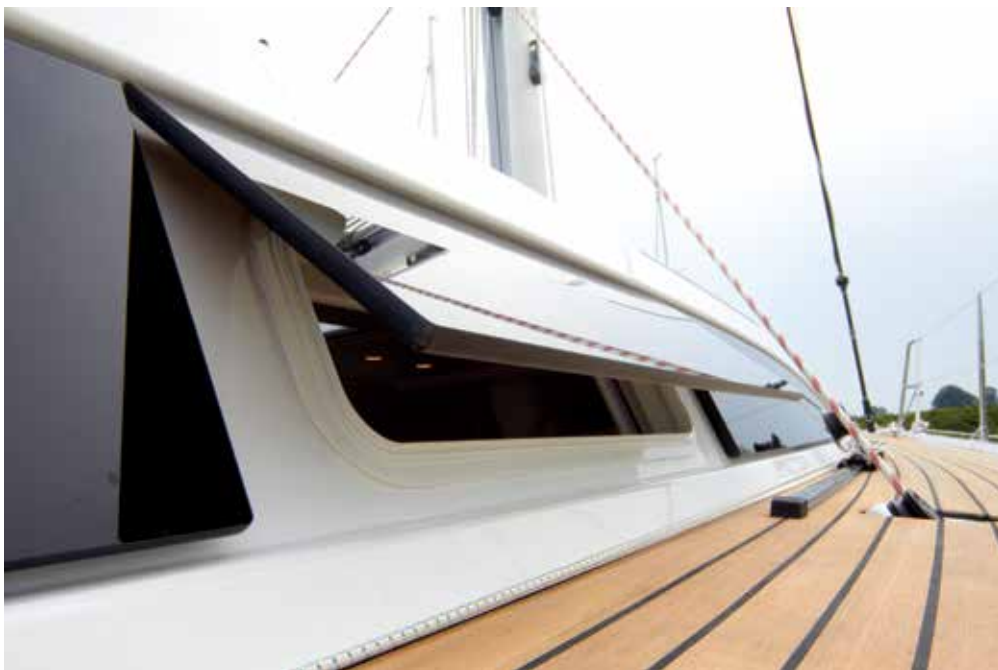
Opening portlight windows and recessed deck fittings
