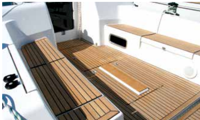
Above: Folding recessed cockpit table
